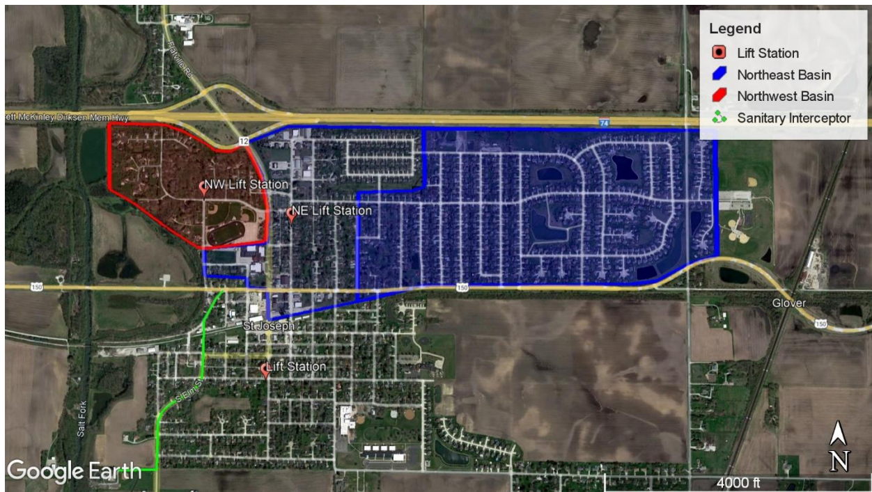
Figure 3. Existing Sanitary Sewer Basins (Northeast, Northwest)
